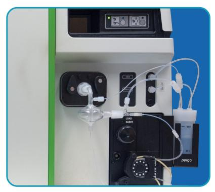
MEINHARD® OneTouch nebulizer includes pre-fitted fluoropolymer liquid and gas lines. Shown installed on NexION 2000 with pergo 2000 AMS.
