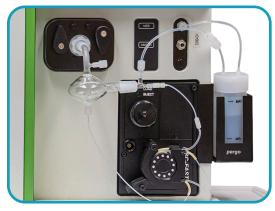
pergo 2000 systems mount onto existing NexION 1000/2000/5000 pumps as well as FAST and prepFAST DXi modules
