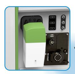
Base Module integrated with NexION 2000 ICPMS PC<sup>3</sup> Peltier Cooler shown but not included
